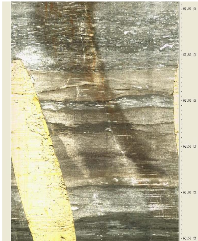
Figure 18. Down-hole camera image (360-degree view) showing dyed grout in an intersected grout hole. Depth is 61.0 to 63.5 feet (Source: The Judy Company).
